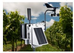
can now receive real-time, site-specific weather data on their smartphone including temperature, relative humidity, rainfall, wind speed/direction and solar radiation.
